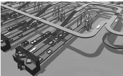
Fast moving items will be automatically moved to locations close to the picking stations to minimise the amount of time it takes to collect the stock for each order.
